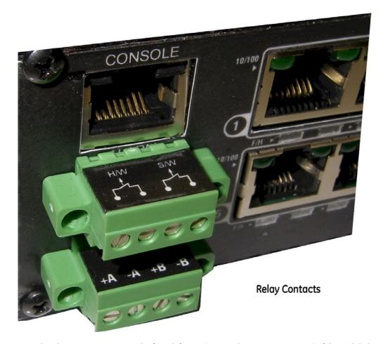
The Alarm Contacts are on the front left area (next to the DC power source) of the Multilink ML1200 unit and are green in color as shown in the picture.
